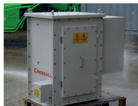
Cressall ATEX neutral earthing resistor (NER) undergoing an IP-water test.
