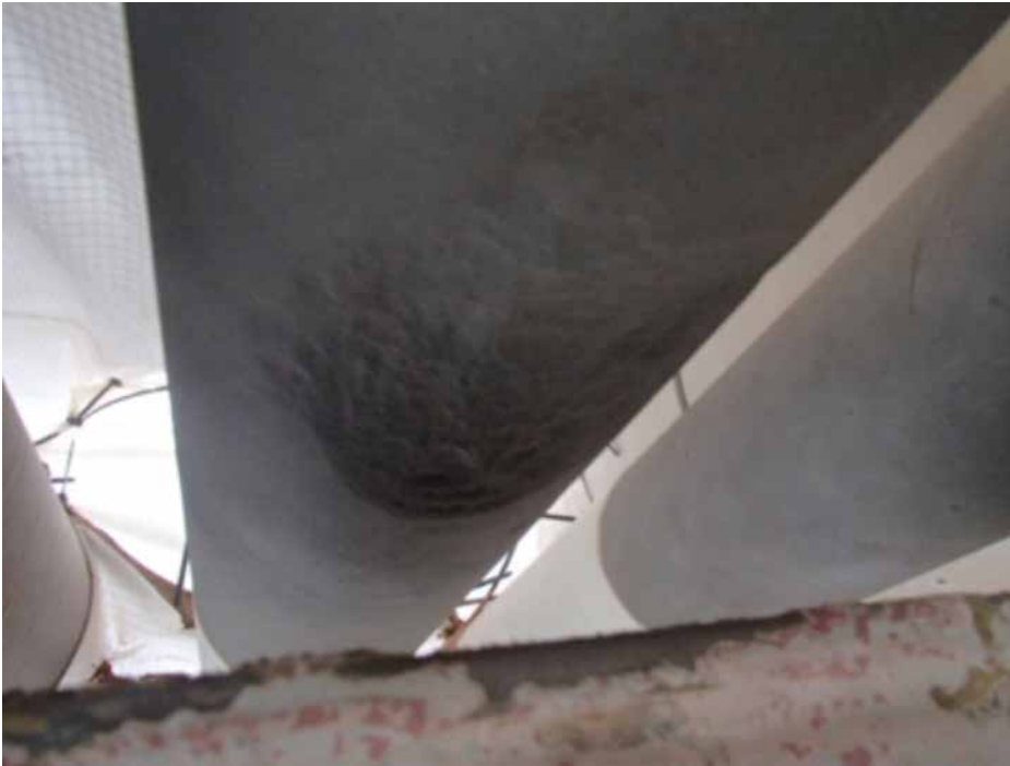
Above: Thin-wall corrosion up to 35%
